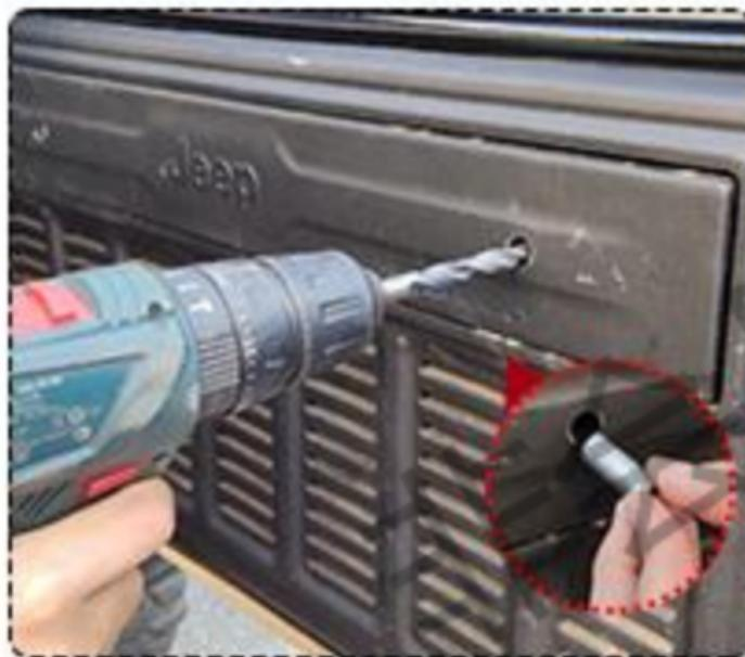
After drilling a 13mm hole, place a small circular slider
