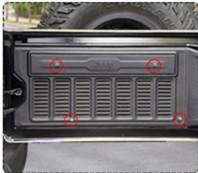
Remove the tailgate panel, locate and mark the original four hole positions
