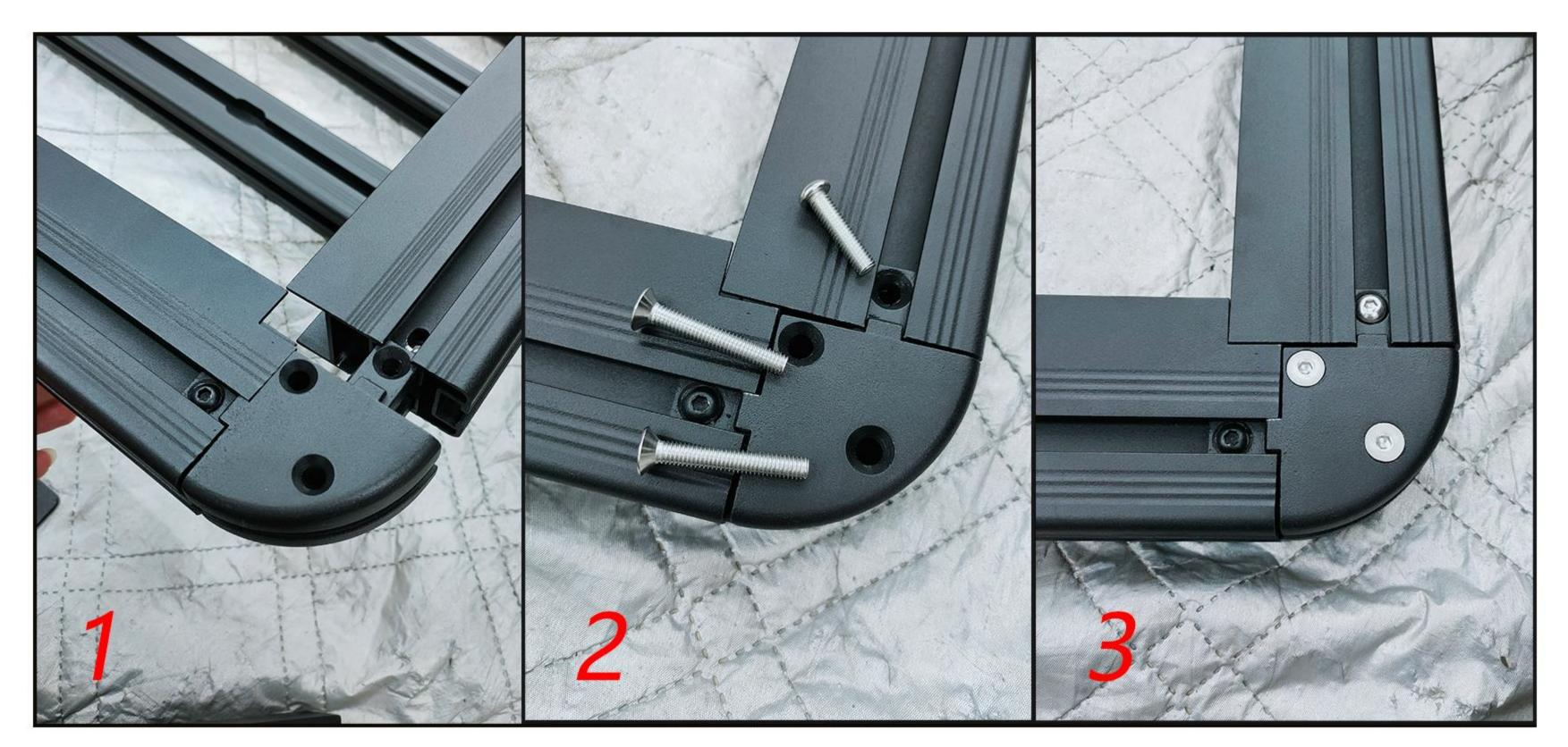
Butt joint of one side luggage rack cross bar (As figure 1 2 3). Another side cross bar should be installed after the middle crossbar is placed, then tighten screws (As figure 7)
