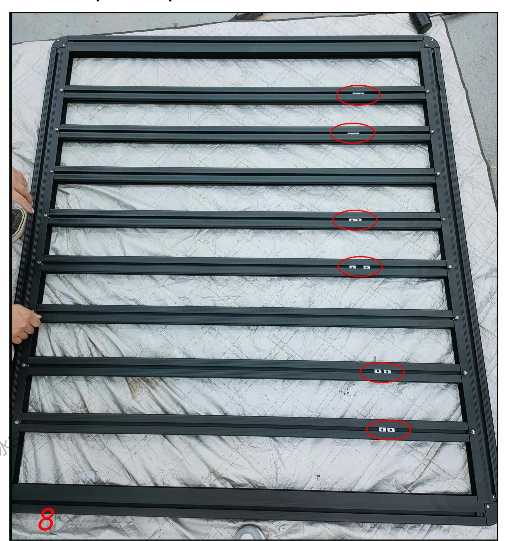
Place Six pieces nuts on the each side of cross bars (Figure 12). Tighten the screws (Figure 13), and install all the brackets (Figure 14)
