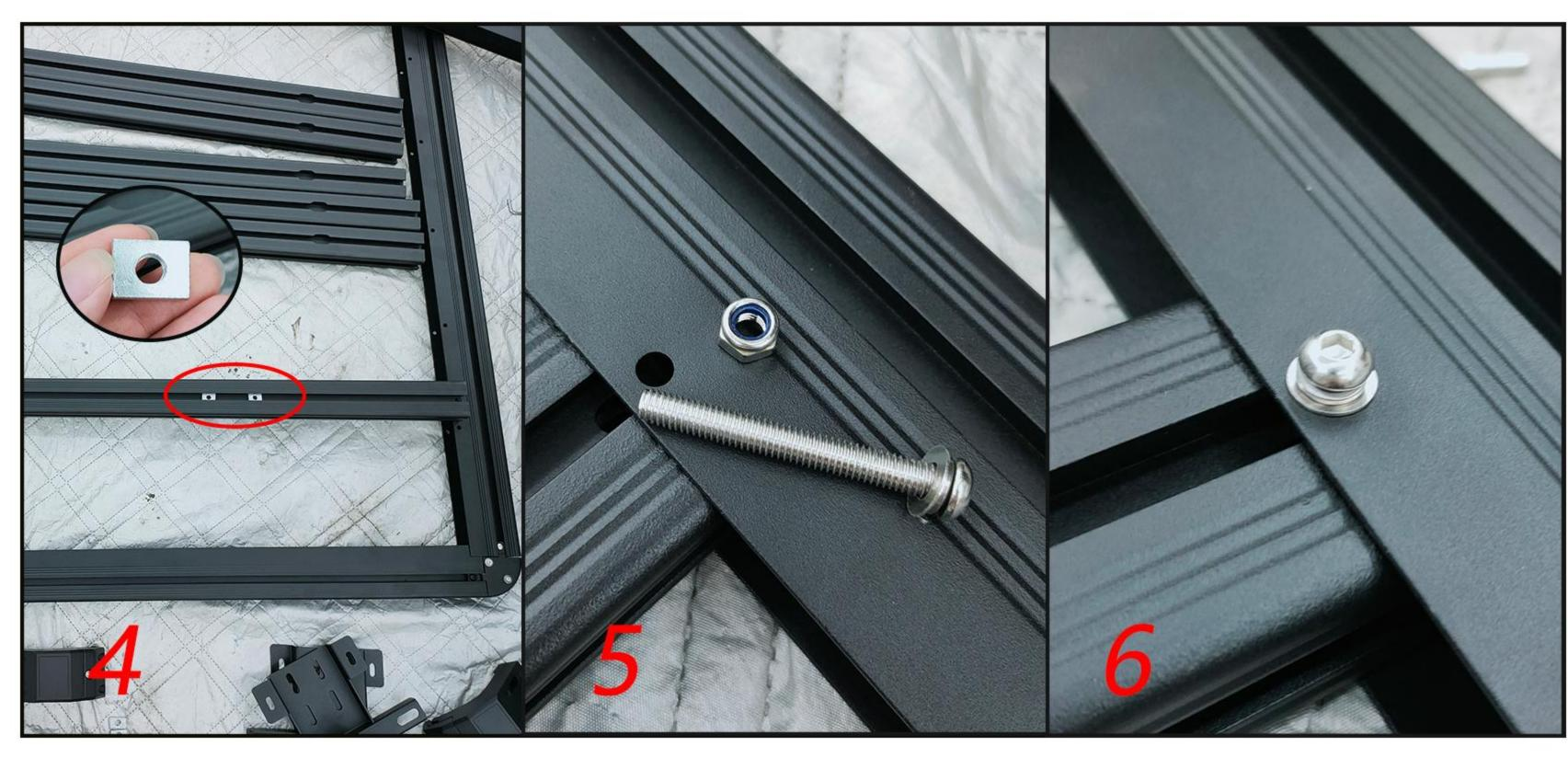
Put the nut into the groove(figure 4),use the screw (figure 5) and tighten(figure 7).Put nuts in the places circled in Figure 8, put 2 pieces in each place, total need to put 12 pieces
