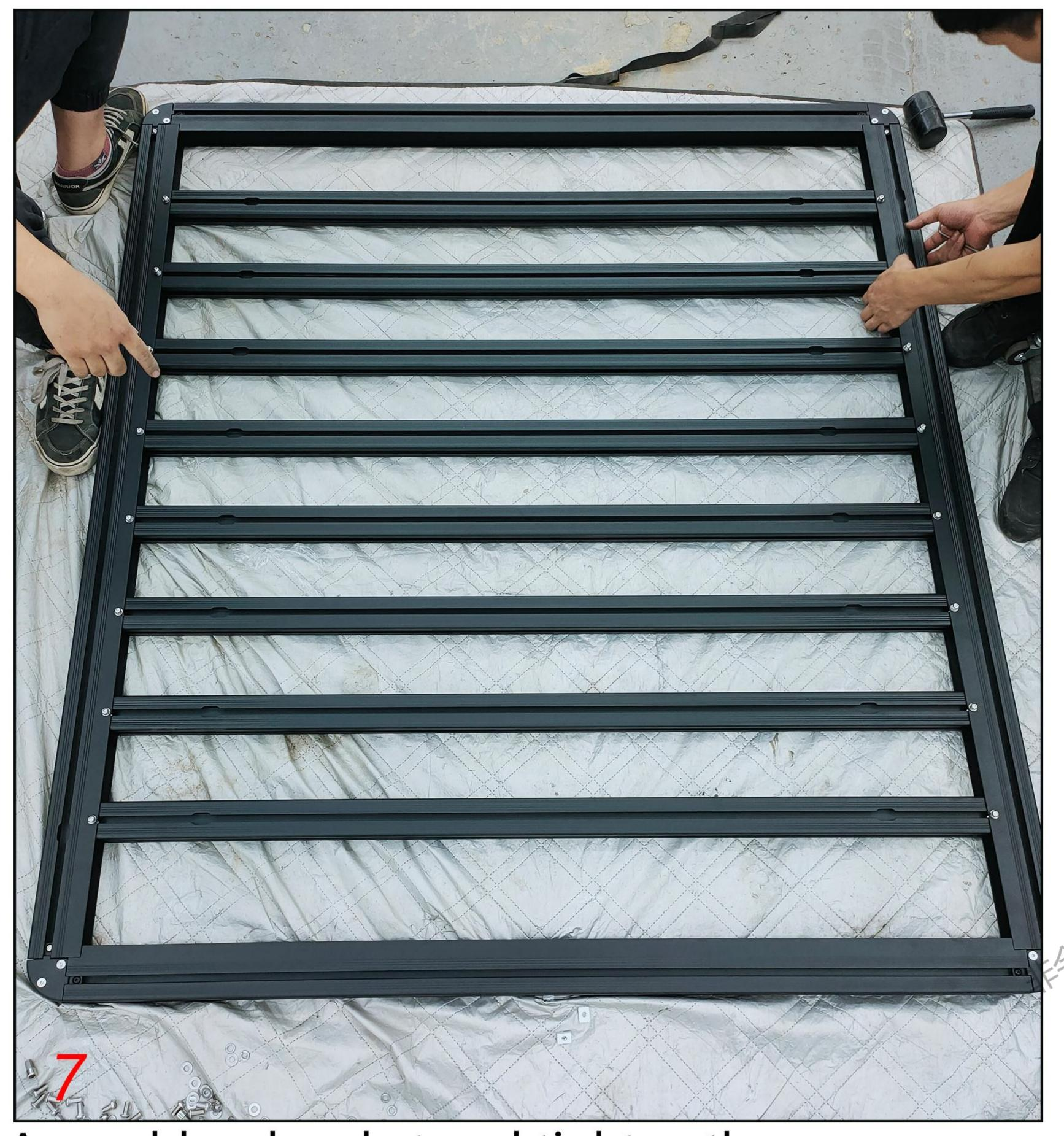
Assemble a bracket and tighten the screws, (note that the bracket should be aligned with the red line in Figure 11)
