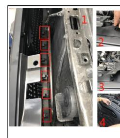
1: Push the grille to the proper buckle position (figure 1)
