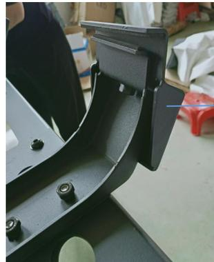
Note: This outer cover is only a flat-bottom installation effect. In actual installation, only the inner bracket needs to be installed. This outer cover is installed and locked after the luggage frame is assembled and moved to the roof of the
